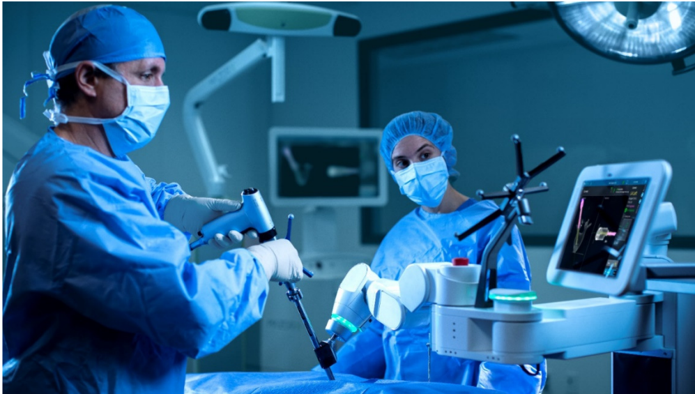
Fig. 2.3 Mazor X StealthEdition™ by Medtronic, a navigation system for spinal and orthopaedic surgery. Surgical instrument localization is achieved by i) robot kinematics and ii) optical tracking of reflective markers. Image source: Medtronic.
